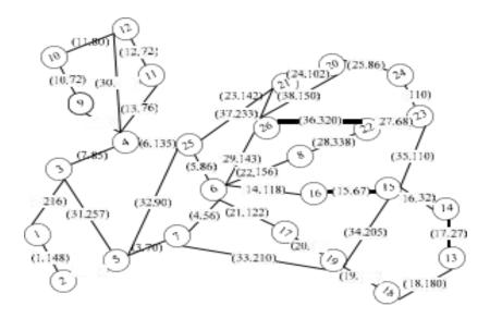
Figure 1: Topology of communication network of the IEEE 30-bus test system.
